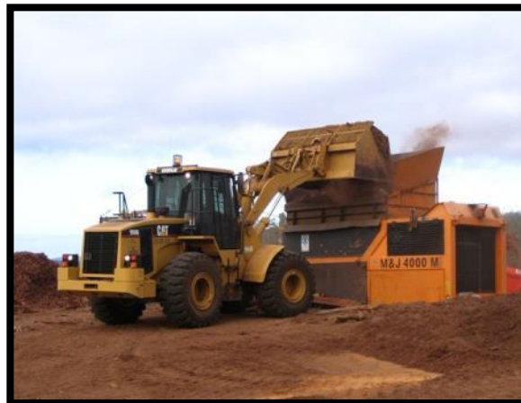
Figure 17: Waste Reducer processing waste wood from bauxite mining
