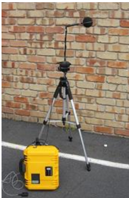
Figure 6: The “Yellow Brick” noise logger and complaint recorder
