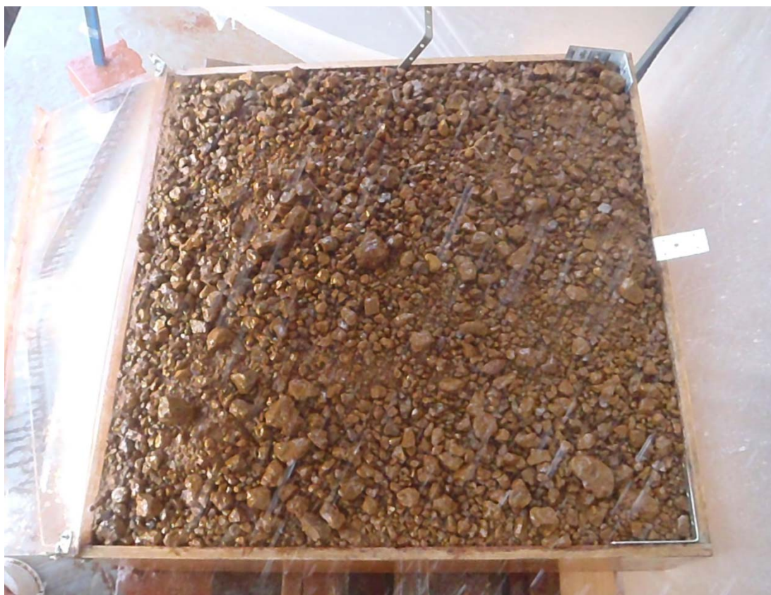
Plate 4.4: Self-armouring of gravelly material during erosion testing
