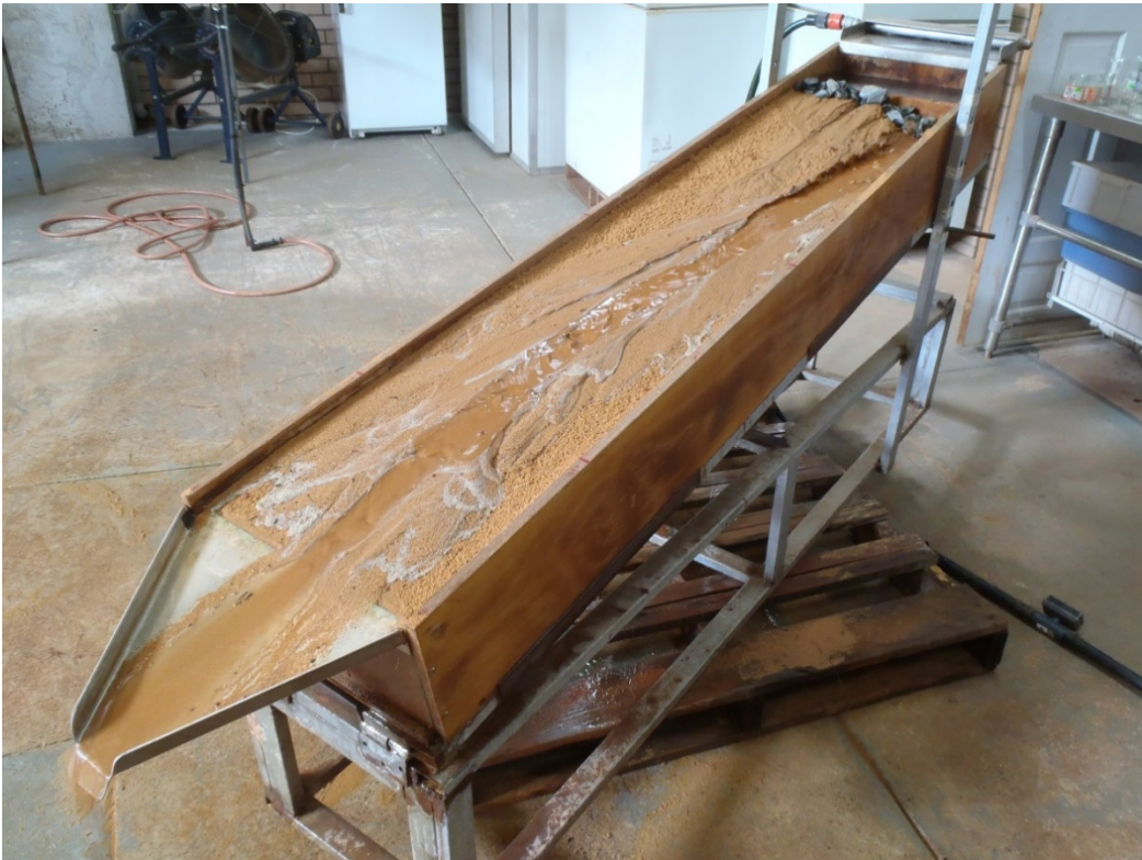
Plate 4.3: Laboratory-scale, rill erosion flume
